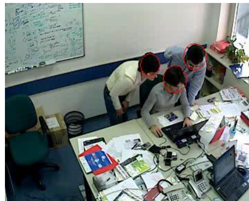
Figure 6: Head detection through ellipse fitting for a group of three persons.
