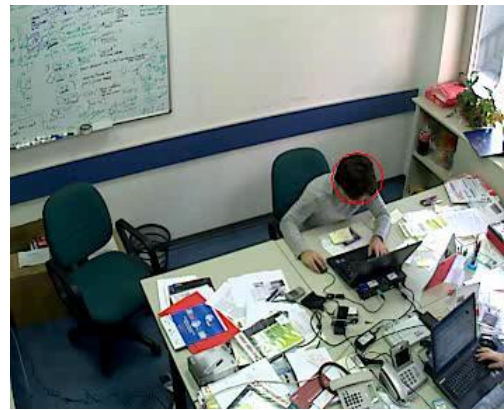
Figure 5: Head detection through ellipse fitting for a single person.
