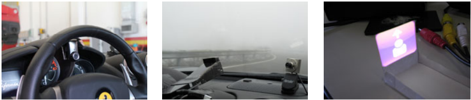
Fig. 1. a, Camera sensor position behind the steering wheel. b, Head-up display projection hardware below the windshield. c, Icon for visualizing the eyes-off-the-road state.
