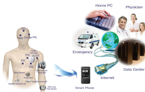
Figure 1: The system model of body sensor networks proposed by the Integrated Microsystems Enterprise (IME) in College of Engineering at Michigan Technological University, USA.
