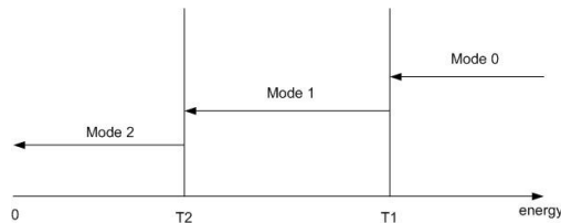
Fig. 3. Power thresholds and modes for power management
