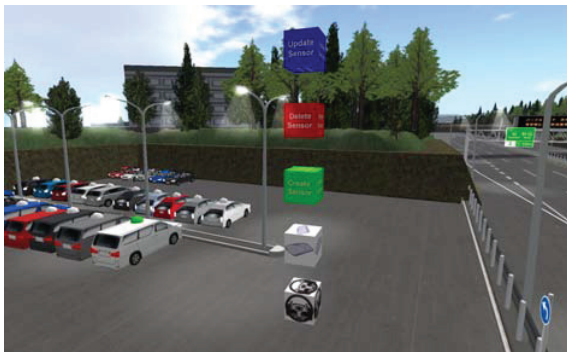
Figure 4: A button array interface displays the menu of options for sensor manipulation (top three buttons) and user driven vehicle instantiation (two buttons at bottom).
