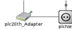
Figure 3. Compound module consisting of a socket adapter modem (see figure 2) and a network management module
