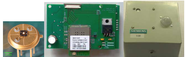
Figure 4. Gas sensor (left), gas sensor module board (middle), and housing (right) as implemented in the SmartSenior project
