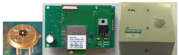
Figure 4. Gas sensor (left), gas sensor module board (middle), and housing (right) as implemented in the SmartSenior project
