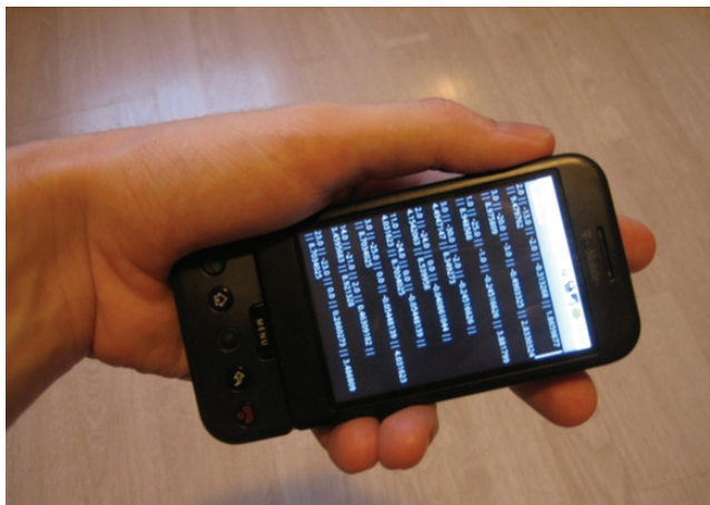
Figure 2. An experimental session with DroidGlove on a HTC G1 smartphone: debug information about acceleration and orientation is reported in real-time on the screen.
