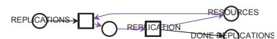
Figure 10: Job computation workflow representing replications as tokens rather than explicit paths in the workflows. Parallel execution of replications is given when resources (cores) are available in the resources place and a replication token is available.
