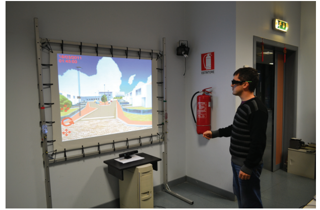
Figure 7: Navigation of a digital site through body poses. The stereoscopic 3D vision is provided by shutter glasses worn by the user.
