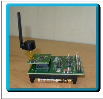
Figure 4. Battery powered anchor node
