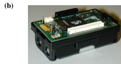
Figure 1. a) Wireless sensor “nodes” or “motest,” b) practical size of 2 cm 3
