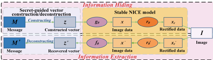
Fig. 1. The framework of SM-IG scheme for generative steganography based on the Stable NICE model.
