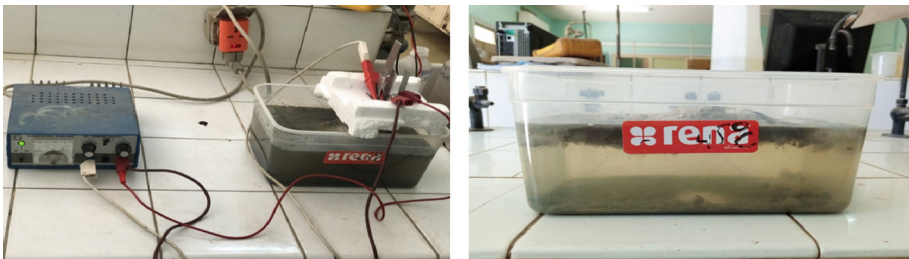
Fig. 5. Electrocoagulation reactor before and after treatment
