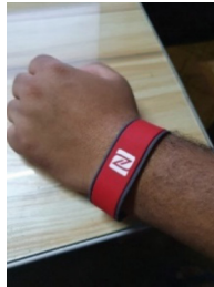
Fig. 2. NFC Chip embedded in Silicone Bracelet
