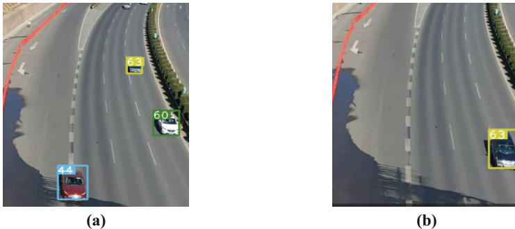
Fig. 5. Vehicle tracking detection effect of (a) the current frame and (b) the next frame.
