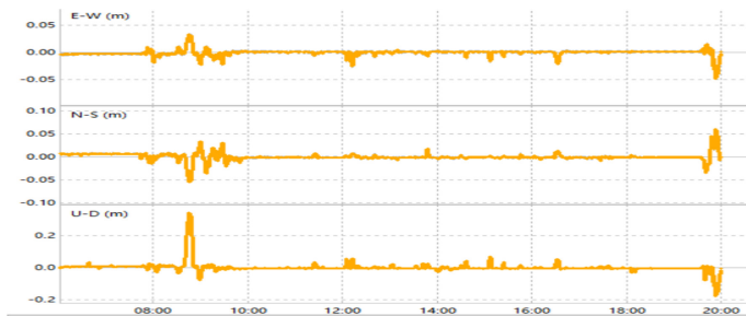
Fig. 2. Distribution of the RTK positioning Result at DUCH
