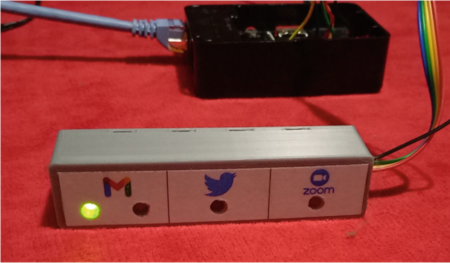
Fig. 9. Green LED switches on when there are no unread emails
