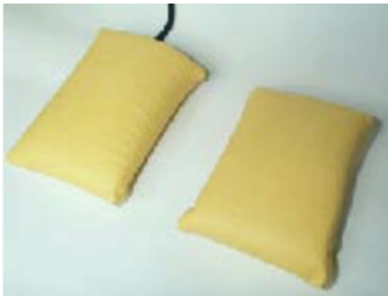
Fig. 1. Metal plate electrodes covered by fabric tissue.
