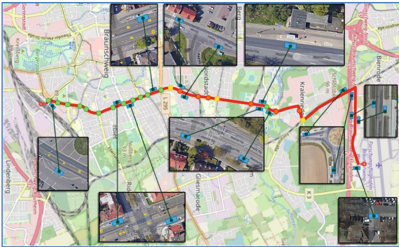
Fig. 7. Overview of the mobility corridor as a test field for the demonstration and management of virtual stops in Braunschweig, Germany. (Color figure online)
