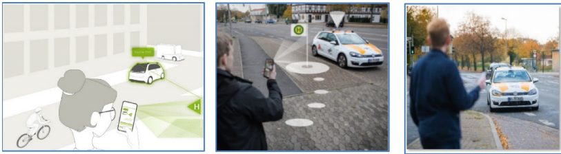
Fig. 6. DRT end user using prototype AR app for the localization of the virtual stop at the pick-up location (source: DLR).
