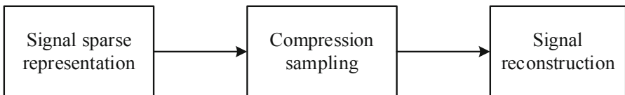
Fig. 1. The processing of compressed sensing
