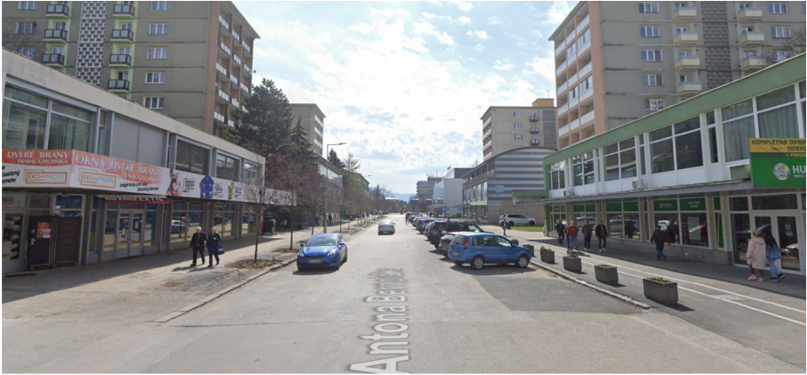
Fig. 2. Picture of the part of the measurement area. Canopies sheltering part of the sidewalks on both sides of the street challenge the reception of GNSS and cellular network signals.
