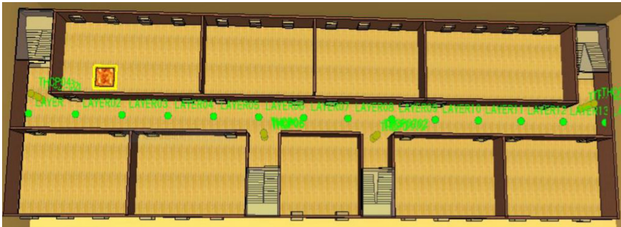
Fig. 4. The setting of thermocouples
