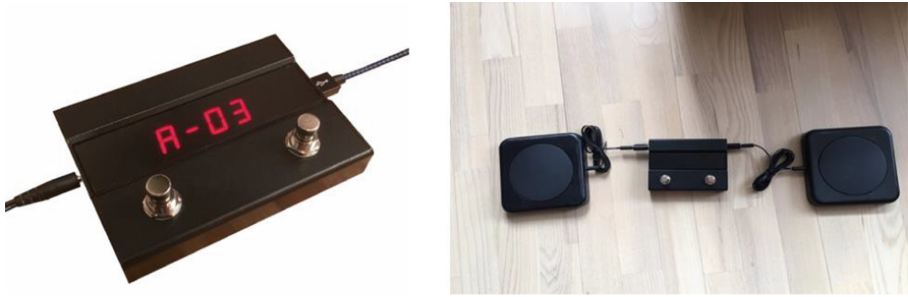
Fig. 3. (Left) Optional aFrame switch = bank and patch change of sounds [with permission ATV] (right) supplemented with two adaptive switches each side for easier operation by users having hand weaknesses. These are input-output devices that allow individuals with physical disabilities to independently activate devices such as the aFrame
