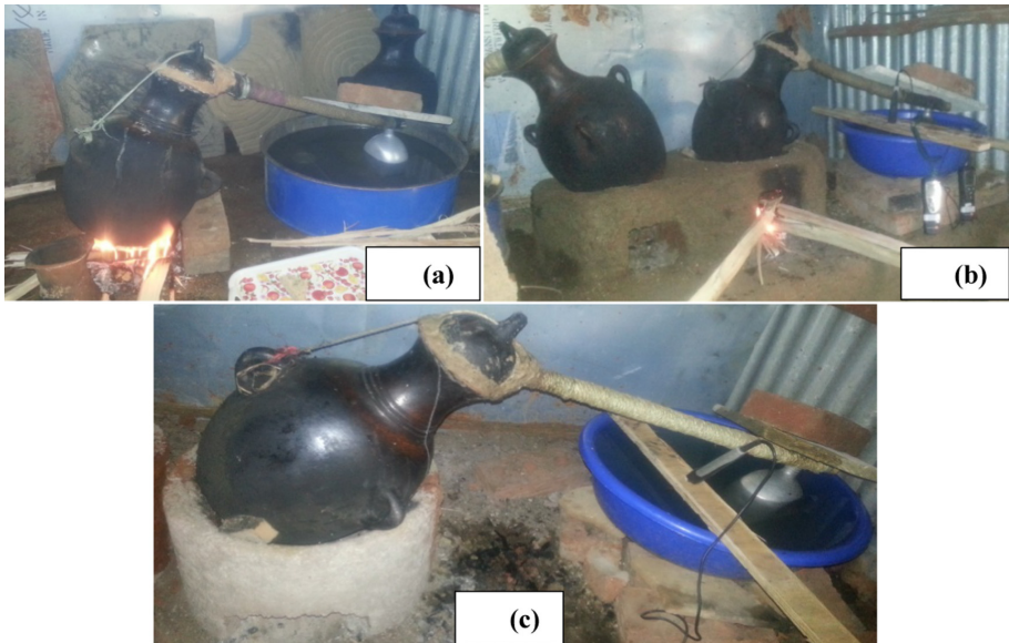
Fig. 3. Areke stoves: (a) three-stone fire, (b) traditional and (c) Mirt Areke
