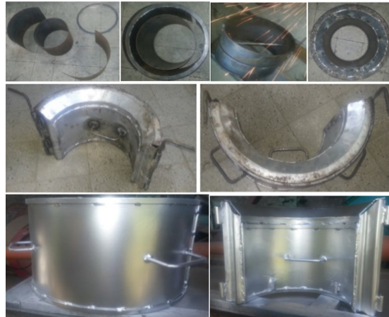
Fig. 2. Final mold for Mirt Areke Stove
