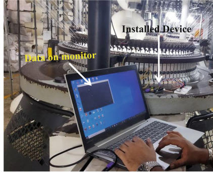
Fig. 2. Parts of the knitting machine’s basic components and experimentation on the weft circular knitting machine
