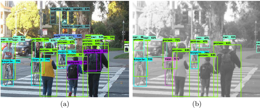
Fig. 7. Visual impact on object detections before and after the application of tuning knobs. (a) unmodified video frame and (b) video frame after applying knobs - colorspace modification, denoising, contrast stretching and gaussian filtering.
