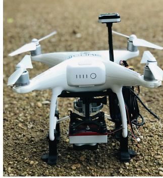
Fig. 2. MicaSense RedEdge-MX camera mounted on a DJI Phantom 4 drone.
