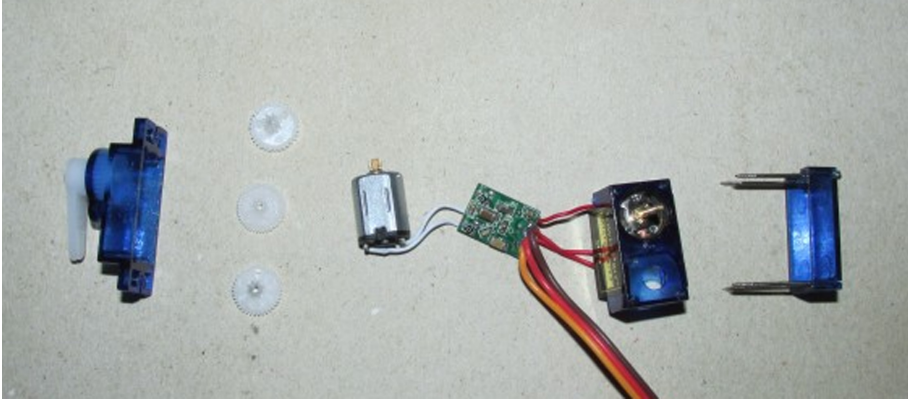
Fig. 4. The various constituents of SG90.
