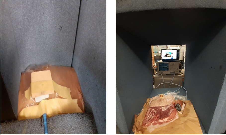
Fig. 7. UWB measurement setup inside the cube made from absorber pieces [3].
