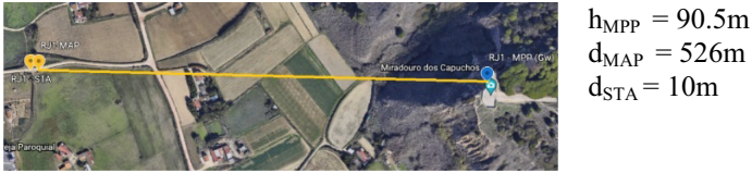
Fig. 14. Test B: map view (google maps), h_{MPP} and link distances.
