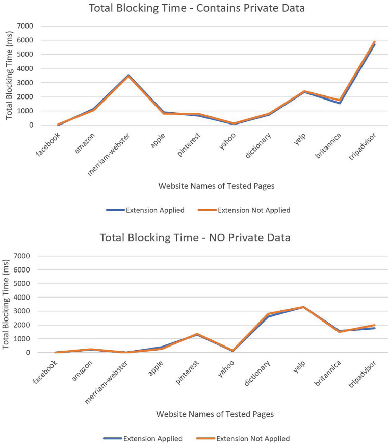
Fig. 8. Total Blocking Time measurements for web pages that contain private data and those that do not contain private data.
