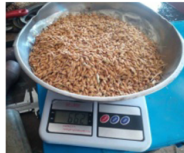
4f. Sample weight measurement of cleaned grain for performance analysis
