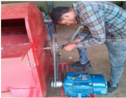
4c. Drum speed measurement using tachometer
