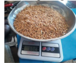
2d. Sensitive digital Weighing Scale (Sensitivity: 0.1 g)
