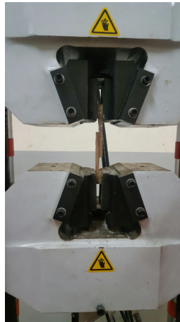
Fig. 4. Tensile testing machine, UTM: WAW-600D
