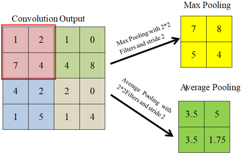
Fig. 5. Examples of max pooling and average pooling
