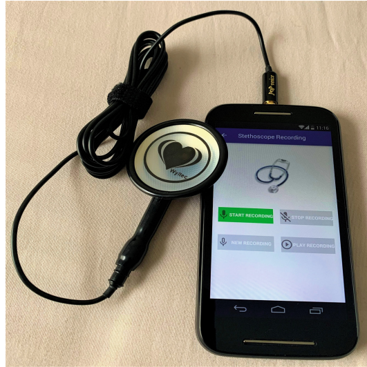
Fig. 1. The Audio-Technica ATR-3350IS omnidirectional condenser lavalier microphone (with heart shape on surface) connected to the Motorola Moto E smart-phone device to collect breath sounds from COPD patients. The custom mobile application is shown on the screen of the smart-phone.
