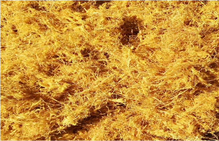
Fig. 3. NaOH (10 Vol%) and corn starch soaking treated bamboo fiber.
