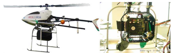
Figure 5. The Hirobo Freya EX 90 RC helicopter and its computer system (PC-104)
