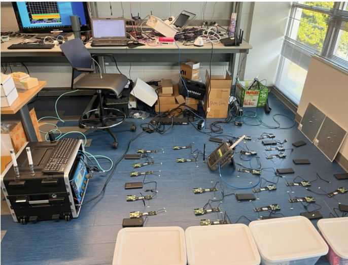
Fig. 2. In lab testing with low-cost U-NII-4 interferers
