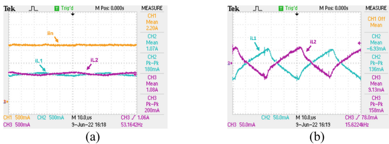
Fig. 10. Experimental results of the PI algorithm with a reference current of 2.25 A: (a) Average value of the currents in each arm, i_{L1} and i_{L2} , and at the input, i_{in} ; (b) Ripple of the current on each arm, i_{L1} and i_{L2} .
