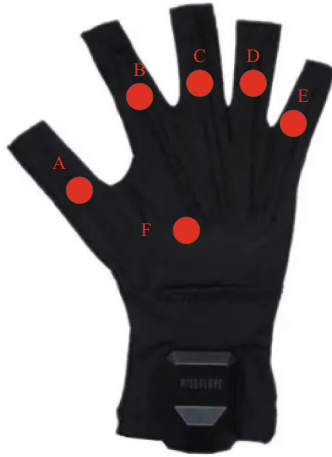
Fig. 4. 5DT Data Glove Sensor Distribution Diagram
