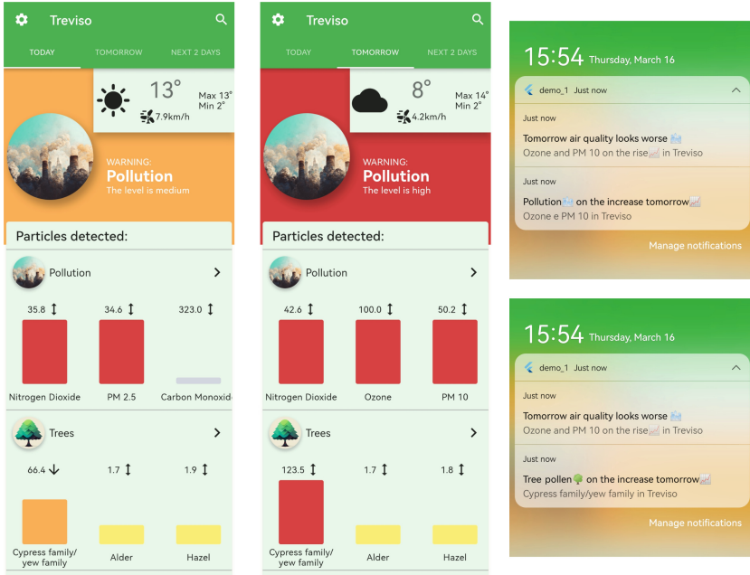
Fig. 4. Particle levels today (left) and tomorrow (center) in Treviso, notification when diary is empty (upper right) and when cypress family is in the diary (lower right)
