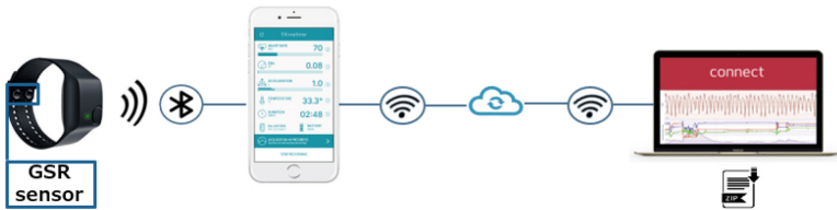
Fig. 2. The E4 IoT-enabled GSR data acquisition process: following the measuring session, data can be retrieved from the Empatica cloud platform.
