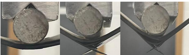
Fig. 6. The process of three-point bending test
