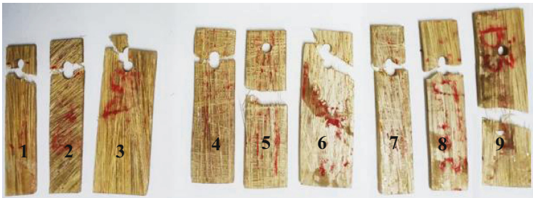
Fig. 9. The failure mechanisms of single lap bolt joint DPFRPC
