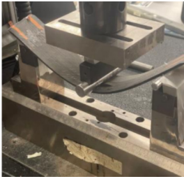
Fig. 4. Three -point bending test.
