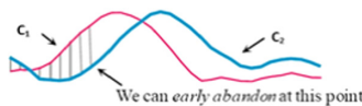
Fig. 1. An illustration of early abandoning in calculating Euclidean distance between C_1 and C_2 .
