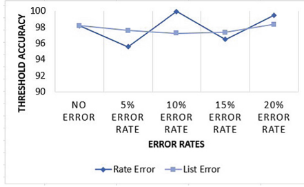
Fig. 9. Accuracy of leakage detection in HPN
