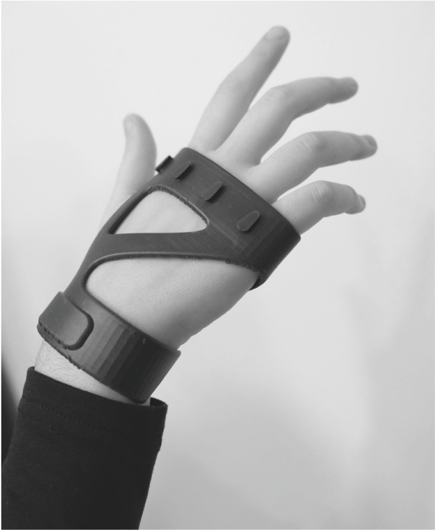
Fig. 5. Prototype of the therapeutic device worn. As you can see from the image, the adherence of the device to the user's hand is perfect, this is due also to the use of digital modeling and advanced prototyping techniques.
