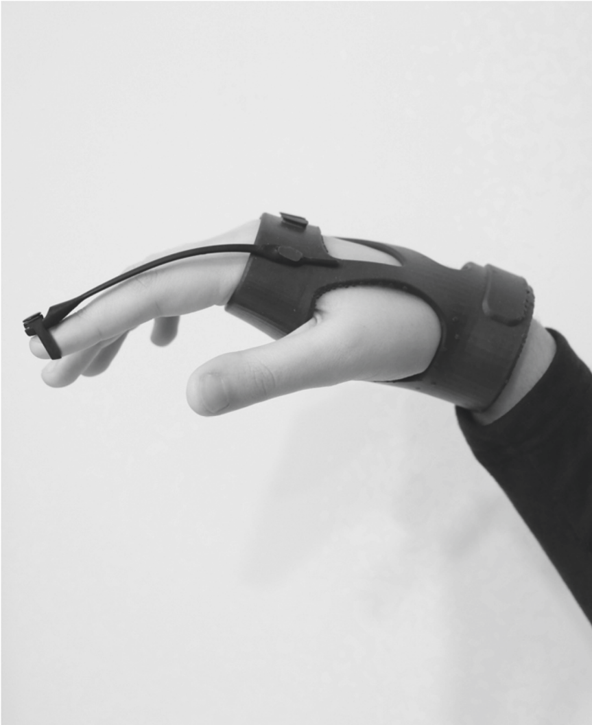
Fig. 6. Prototype of the therapeutic device worn. In this image it is possible to see the integration of flexible elements necessary for carrying out the therapy.
