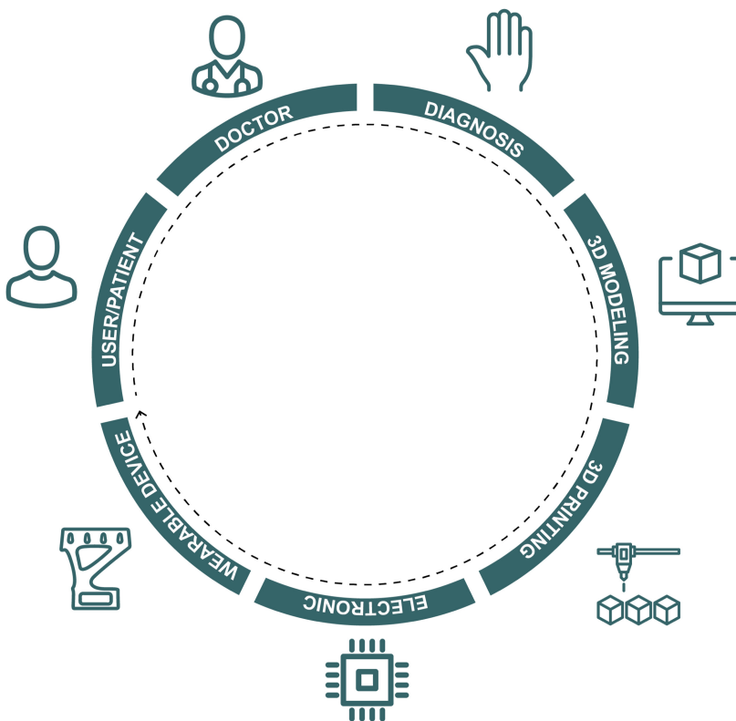
Fig. 2. Design model: the patient addresses the doctor who carries out the collection of anthropometric data and assigns the most suitable therapy. The data is used to three-dimensionally tailor-made the device, which is then 3D printed. The components necessary for the operation of the device are then added to the printed object. Once completed, the device is ready to be worn by the user and used.
